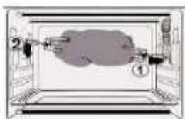
Insert the rotisserie forks in the rotisserie orifice and then place the drip pan under the rotisserie
