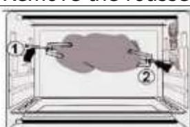
Remove the rotisserie forks using the rotisserie handle and then remove the drip pan
