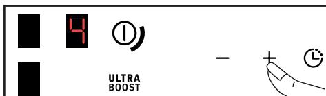
With a power < 5, a quick double press on the + button allows direct access to power 5.
