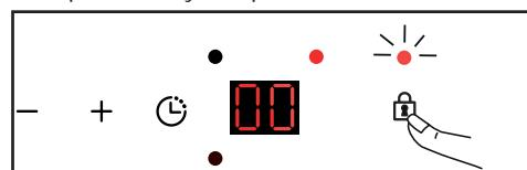
The display of cooking zones in operation alternately indicates power and the locking symbol .
