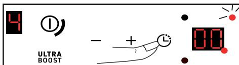
The timer zeros are flashing with the timer units LED and the active focus LED.
