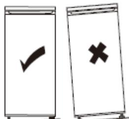
If the appliance is not level, the doors will not be correctly aligned and compartment sealing will not be ensured.
