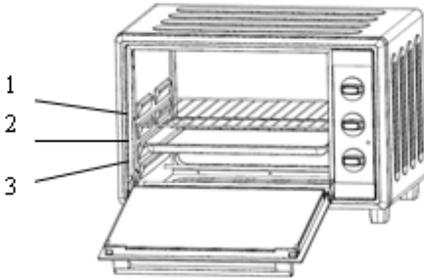
There are 3 different positions for the tray which you can adjust according to the dish you are cooking. For example, when cooking macaroni gratin, to have the top part cooked the most, use the third position. For roasting a chicken, use the first position.
