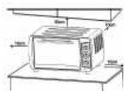
If the oven is placed too close to a wall, the wall may become burned or discoloured. Ensure that curtains, etc. are not in contact with the oven.
