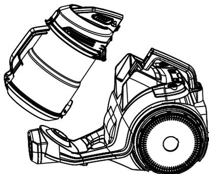
2. Put the dust cup onto the rubbish bin, push the release button to open the bottom cover of the dust cup, and the dirt and dust will fall into the bin.
