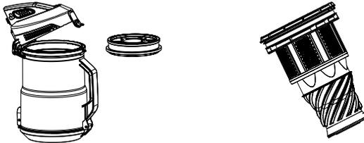
4. Wash the HEPA filter cover, the HEPA assembly, the outlet sponge and the dust chamber in water without detergent and dry them before use. Don't use any tools to brush the HEPA filter, otherwise the HEPA filter will be damaged and filter performance will be affected.
