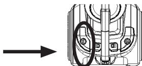
Adjusting the vacuum power : repeatedly press the speed increase and decrease buttons on the socket.
