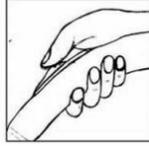
5. Cord rewinding: You can pull the power cord out of the appliance and stop it when you see the yellow mark. Make sure the red mark is not pulled out. When finishing vacuuming, first turn off the power, pull the plug out of the socket, and then press the cord rewind button until the cord is completely in the appliance.
