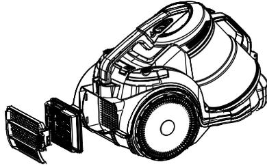
3. Open the dust cup cover and remove the HEPA filter cover and then remove the HEPA filter. Tap it to remove the dust. Rinse it under running water if necessary.
