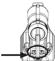
\* You can quickly reduce the suction power by pushing the airflow regulator on the hose handle.
